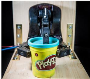
Fig. 1: Using reinforcement learning and tactile feedback, a rolling primitive can be learned on an under-actuated robot hand.
